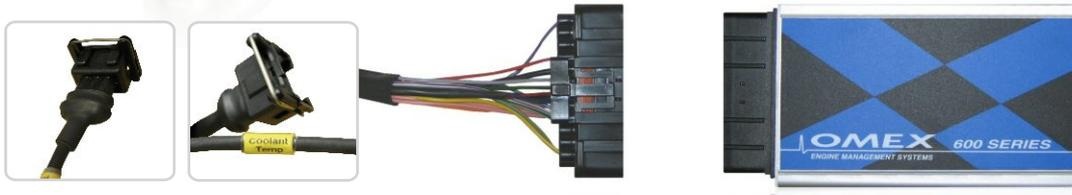
Omex's multi-championship winning 600 Series ECU controls the fuel injection, standard Ford distributorless ignition coil pack, and optionally, many other functions around the vehicle. The ECU is connected to the hardware with a complete, ready built wiring harness, which is fully tagged and with the correct connections made for your Zetec engine, ensuring easy clip-on fitment, optimum performance and absolute reliability.
