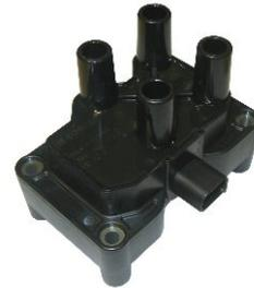
Omex 4 cylinder DIS wasted spark coil pack
