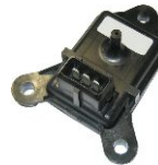
Barometric pressure sensor and harness upgrade
