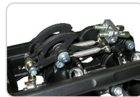
Twin cable throttle linkage kit
