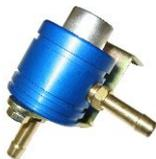
A fixed 3.5 bar fuel pressure regulator in a billet machined aluminium housing. Fuel pipe to go between the regulator and the fuel rail is also supplied.
