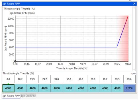
The engine may be able to 'pull through' the ignition retard so also set the Ign Cut RPM table to
