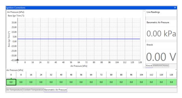
The fuel and ignition can be trimmed to allow for changes in barometric pressure as sensed by a 1bar pressure sensor. The ignition trim is defined in the **Baro Ign Trim table**. The fuel trim values are a known mathematical equation so are inbuilt and are non-adjustable.
