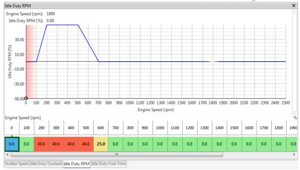
The idle is then fine-tuned and maintained by the feedback loop. **Idle FB- max** and **Idle FB+ max** are the feedback limits for the idle motor. The update rate of this feedback loop is set by **Idle FB Rate**. This would typically be **40**ms with a stepper motor or **200**ms with a PWM device.
