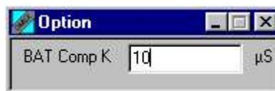
$$\text{Battery Comp Factor} = \text{Battery Comp table value} \times \text{Bat Comp K option}$$
