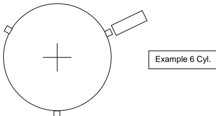
To position the sensor and disc, firstly rotate the engine to approximately 60 degrees BTDC. Then choose where the sensor is to be mounted. At this position one of the lugs on the timing pulley must be facing the sensor. The timing disc is then fixed in that position.
