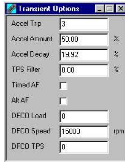
The fuel map contains the fuel for steady state running. Fuel transients such as acceleration and deceleration of the engine especially at gear changes will require different fuelling. To prevent excessively lean or rich stumbles and emission control problems the ECU has two functions; Deceleration fuel cut-off (**DFCO**) and throttle triggered acceleration fuel enrichment (**Accel Trip, Amount & Decay**).
