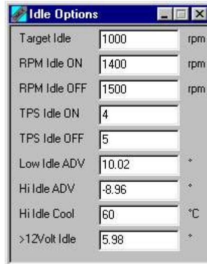
An idle stabilisation algorithm has been included in the ECU to give a stable idle speed by adjusting the idle ignition timing. If the engine falls below the target idle speed, the ignition timing is advanced to accelerate the engine, and if the engine speed is too high the timing is retarded. A good natural idle without the idle stabilisation should be achieved first before enabling the idle stabilisation.
