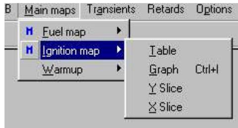
Ignition timing is controlled by a map of numbers. There are 11 load sites and speed sites are at every 400rpm. At each site the timing can be set from 0 to 45 degrees BTDC. Interpolation is used to ensure smooth curves.
