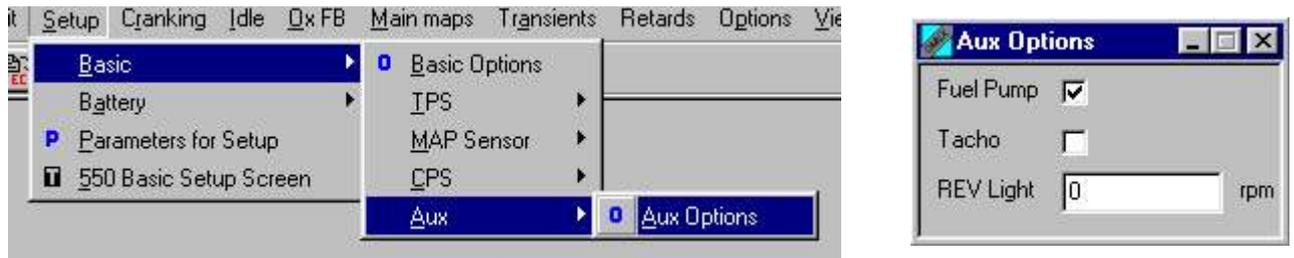
The OMEM550 ECU has a single auxiliary output which can be used as one of three options,
