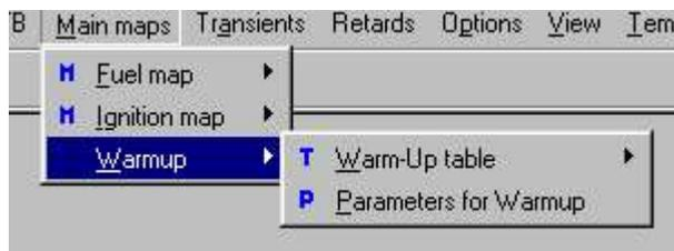
When the engine is cold, it requires an extra amount of fuel. This extra fuel is added as a percentage set in the Warm Up Table of percentage increase against engine coolant temperature.
