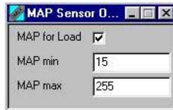
If fitted with a MAP sensor, then the MAP sensor will need calibration. The calibration varies depending on the range of the sensor. MAP sensor ratings are absolute rather than boost pressure so 1bar is for NA engines and barometric compensation, 2bar for up to 1bar boost, and 3bar for up to 2bar boost.
