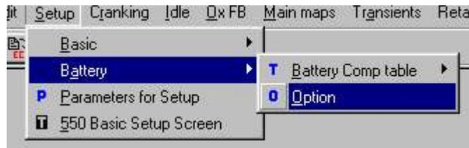
An injection period is made up physically of 2 time periods. The end period is when the injector is open and flowing fuel, but the first period is when the injector is opening its valve and there is no flow of fuel. At low injector durations, this period where the injector is reacting but not flowing fuel can be significant.
