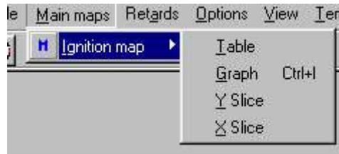
Ignition timing is controlled by a map of numbers. There are 11 load sites and speed sites are at every 400rpm. At each site the timing can be set from 0 to 45 degrees BTDC. Interpolation is used to ensure smooth curves.
